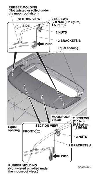
Tighten while applying pressure so that there is no gap between the roof panel and the brackets A and B. Torque the screws to 2.0 N·m (0.2 kgf·m, 1.5 lbf·ft). 15. Remove the shop towels inserted in step 2. Remove the IMPORTANT INFORMATION label.
