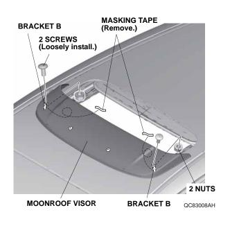
13. Position the moonroof visor with equal spacing in the front and on the sides. Check that the rubber molding is not twisted or rolled under the moonroof visor.
